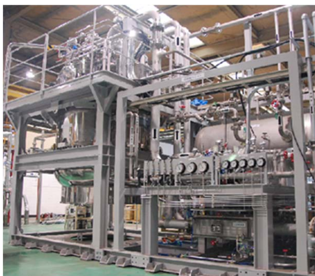
Fig. 2 5kW-class Brayton cryocooler planned for demonstration trials at the Asahi Substation
