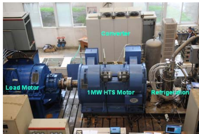
Fig. 5 A view of the 1 MW HTS motor
