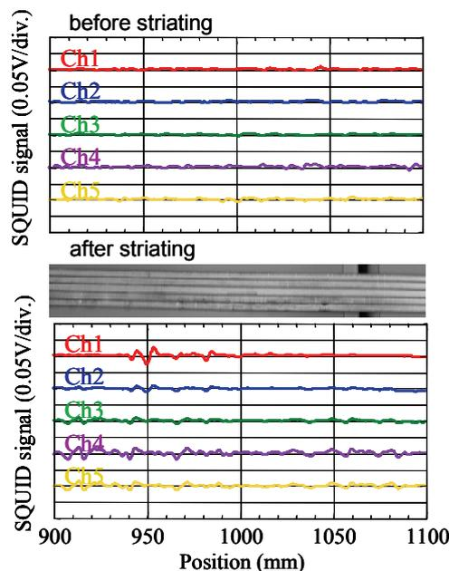
Fig. 3 Example of the superconducting tape evaluation.
