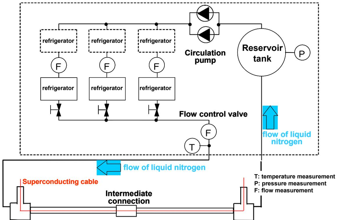
Fig.2 The outline of the entire cooling system verification test
