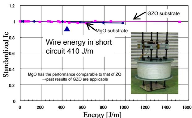
Fig.2 Results of the overcurrent test for MgO substrate wires
