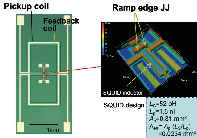
Fig.1 SQUID gradiometer using multi-layer technology
