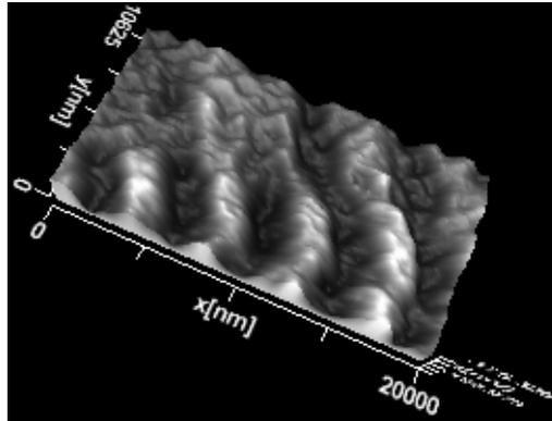
Fig.2 Magnetic image of the hard disk observed by STM-SQUID microscope
