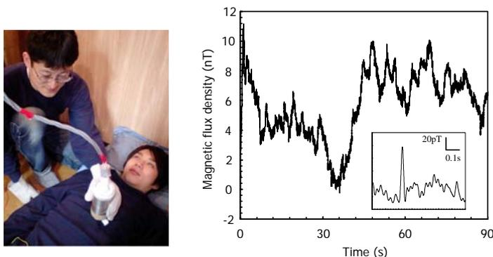
Fig.2 Magnetocardiograms measured with handheld dewar in MSR
