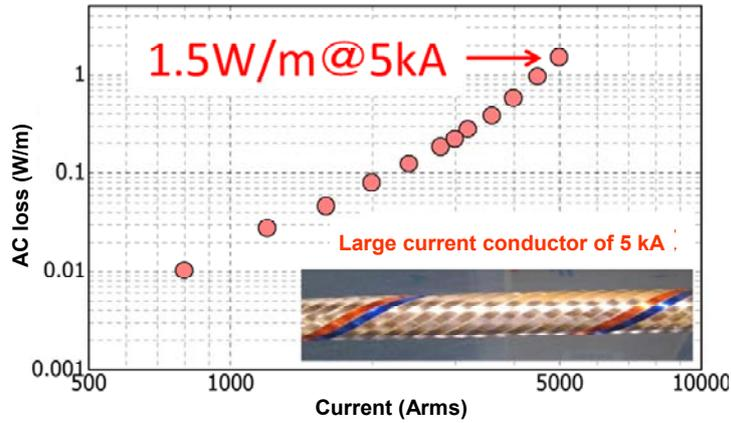
Fig. 2 Measured AC loss of a large current conductor
