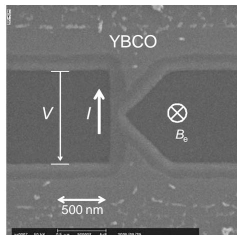
Fig.1 Electron microscope photograph of an asymmetric nanobridge
