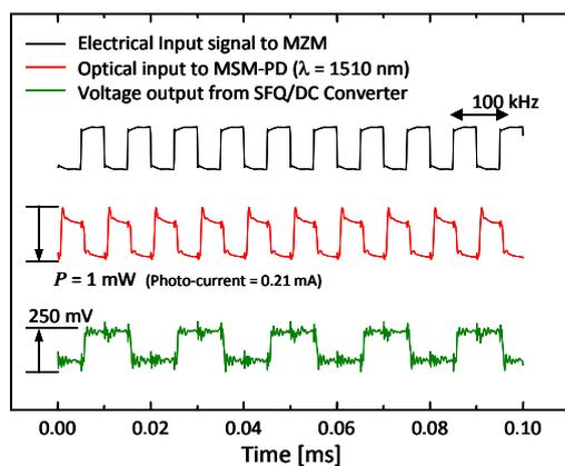
(a) Output waveform for rectangular optical input
