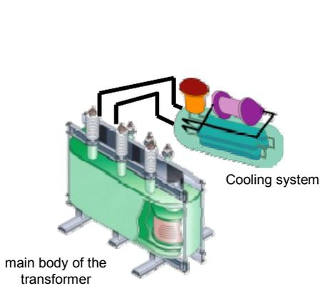
Fig.8 2-MVA transformer model
