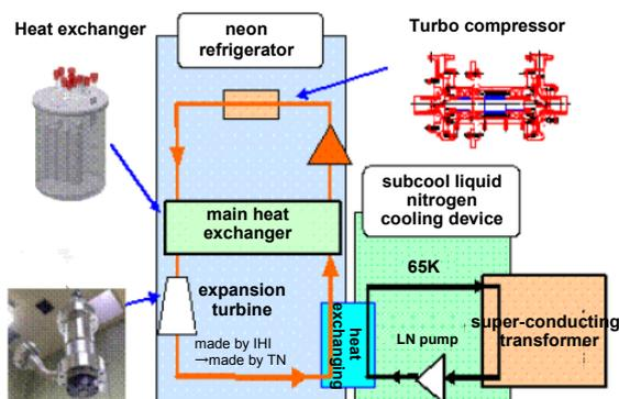
Fig.6 Constitution of cryogenic system
