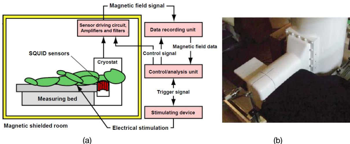
Fig. 1 Constitution of magnetospinography device (a) and appearance (b)
