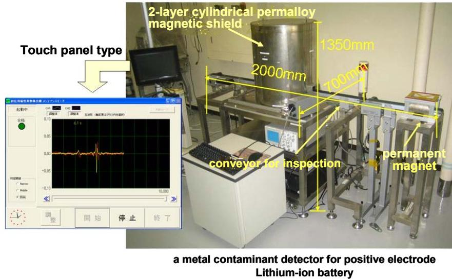
Fig.2 View of the high  $T_c$  SQUID Detection system
