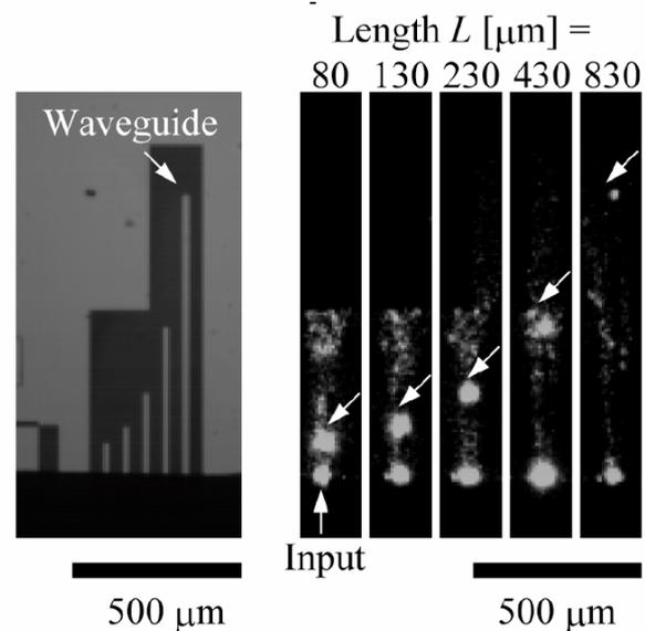
Fig. 2 Metal clad optical waveguide fabricated by using the superconducting integrated circuit process (left-hand side), and the scene of optical propagation in the metal-clad optical waveguide (right-hand side). The way in which the light entering at the bottom of the waveguide moves upward in the waveguide is clearly seen.
