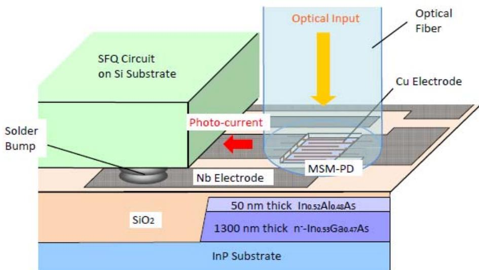
Fig. 1 The schematic diagram of a 1550 nm optical IF module
