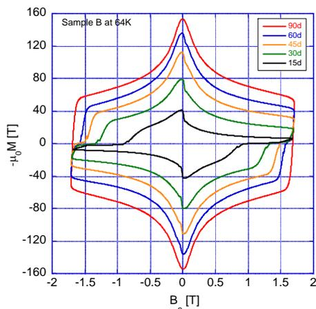
Fig. 1 Magnetizing curve of GdBCO tape wire at 64 K (the magnetic fields are applied at 90°, 60°, 45°, 30°, and 15° to the tape surface)
