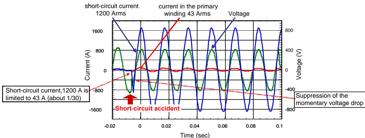
Fig. 5 Test results of current limiting function
