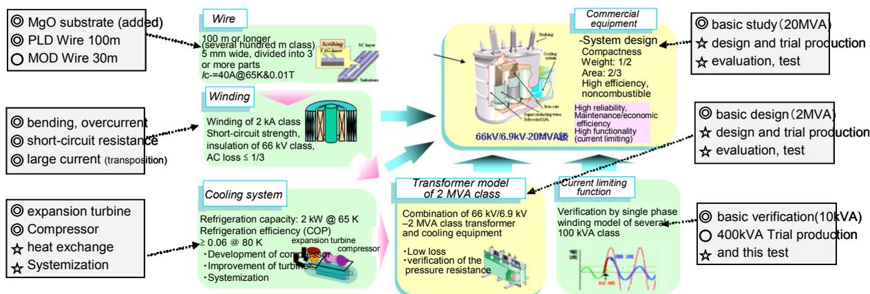
Fig.1 Status of the achievement on the technical development of superconducting transformer (©intermediate target achieved, ○will be achieved within this fiscal year, ☆will be achieved by the end of project)
