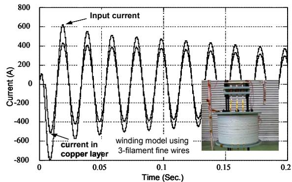
Fig.5 Current distribution characteristics of the winding using fine wires
