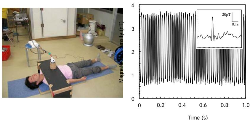
Fig.3 Magnetocardiograms measured with dewar placed on a table outside MSR
