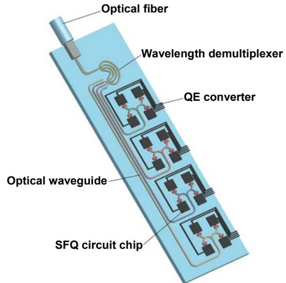
Fig.1 Image of superconducting optical integrated circuit
