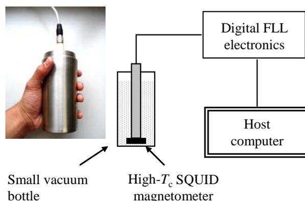
Fig.1 Outline of the handheld SQUID magnetic fluxmeter
