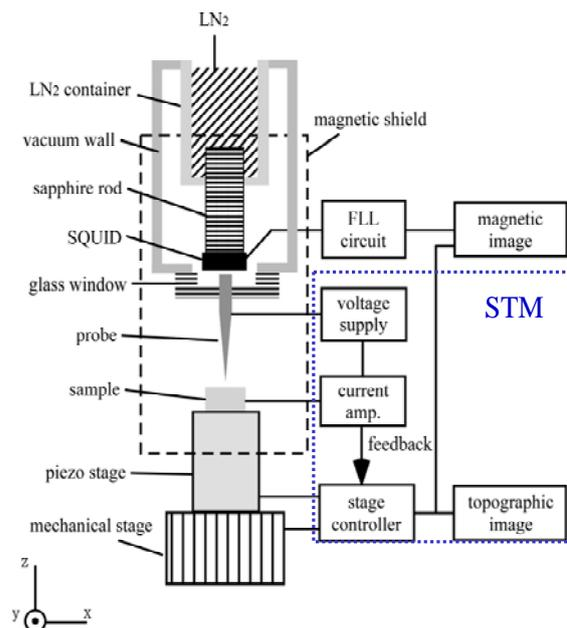
Fig.1 Schematic diagram of STM-SQUID microscope
