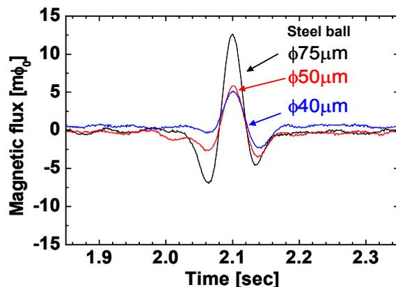
Fig. 4 Time trace of the signals from test steel balls
