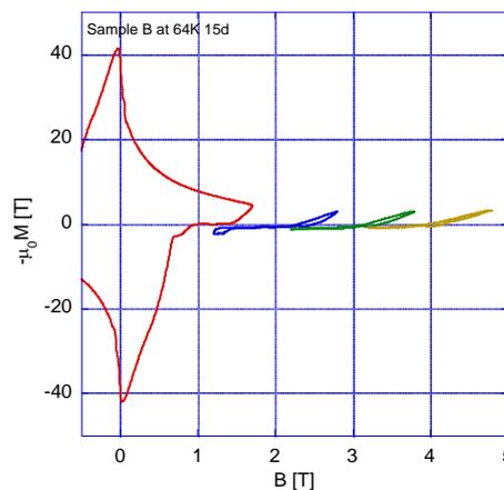
Fig.2 Magnetizing curve of GdBCO tape wire at 64 K (1 in a biased magnetic field based at 15° to the tape surface)
