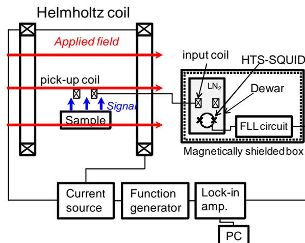
Fig. Non-destructive inspection the system of orthogonally applied magnetic field type using HTS-SQUID
