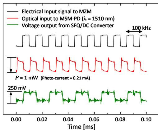
(a) Output waveform for rectangular optical input
