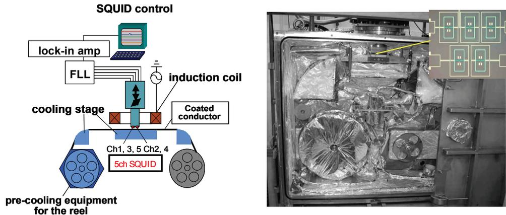
Fig.2 System constitution and photographs of the inside of the vacuum chamber and the gradiometer array
