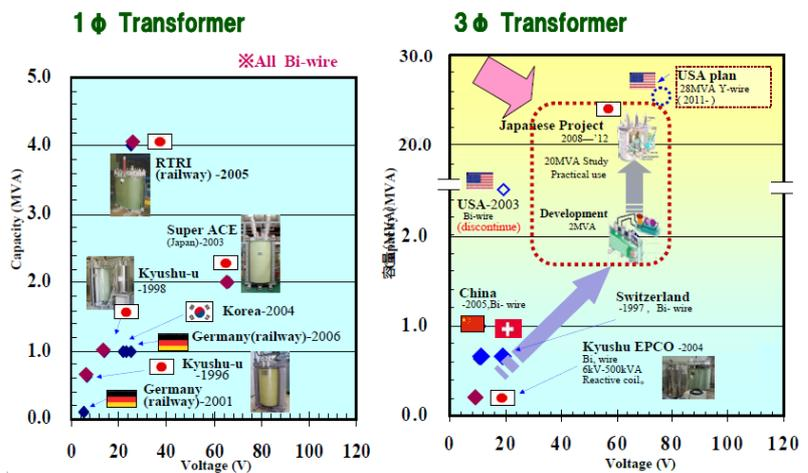
Fig.9 R&D of HTS-Transformer in the World
