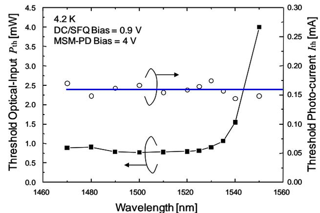
(b) Wavelength dependency of the optical pulse required for the generation of SFQ pulse
