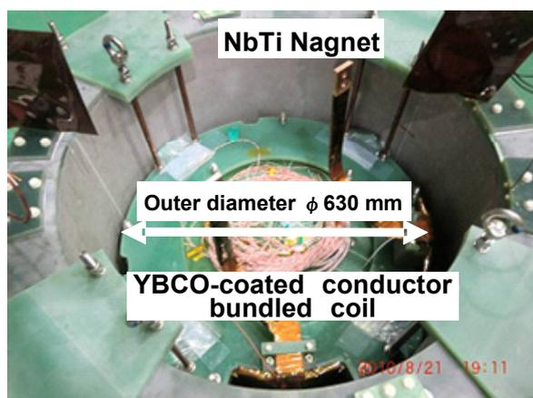
Fig.1 High-hoop-stress test (YBCO-coated conductor bundled coil inserted in NbTi backup magnet, tested at 4.2 K)
