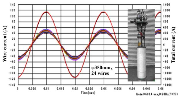
Fig.4 Current distribution characteristics between the wires of the 4-transposition homogeneous current model
