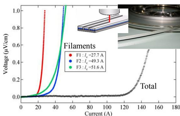
Fig.3 Results of  $I_c$  measurement (PLD wire) before and after thinning the wire
