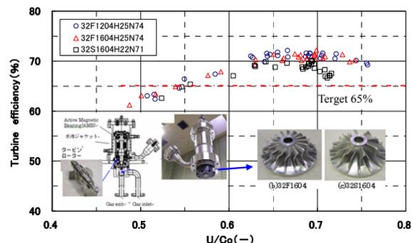
Fig.7 Characteristics of the non-sliding expansion turbine
