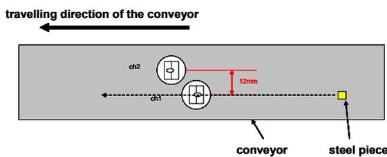
Fig. 3 Top view of detecting section
