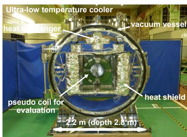
Fig. 2 Cooling system for SMES coil
