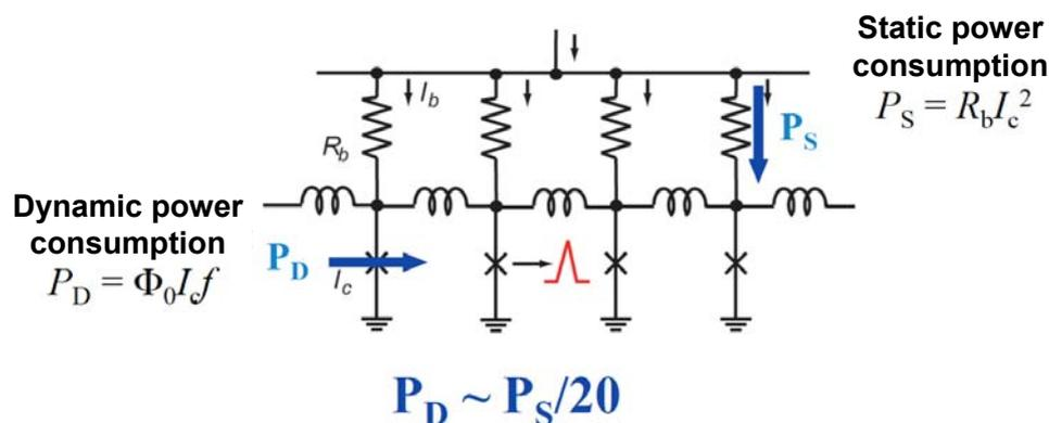
Fig.1 The power consumption of conventional single flux quantum (SFQ) circuit, consisting of static power consumption consumed by the bias circuit and the dynamic power consumption consumed by the Josephson junction itself.
