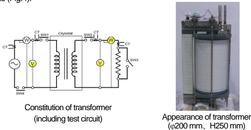
Fig. 4 Y-based small transformer with FCL function
