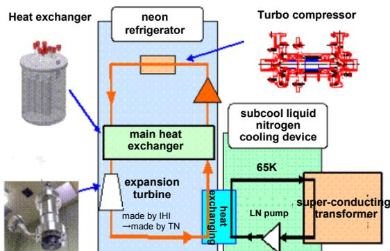
Fig.6 Constitution of cryogenic system
