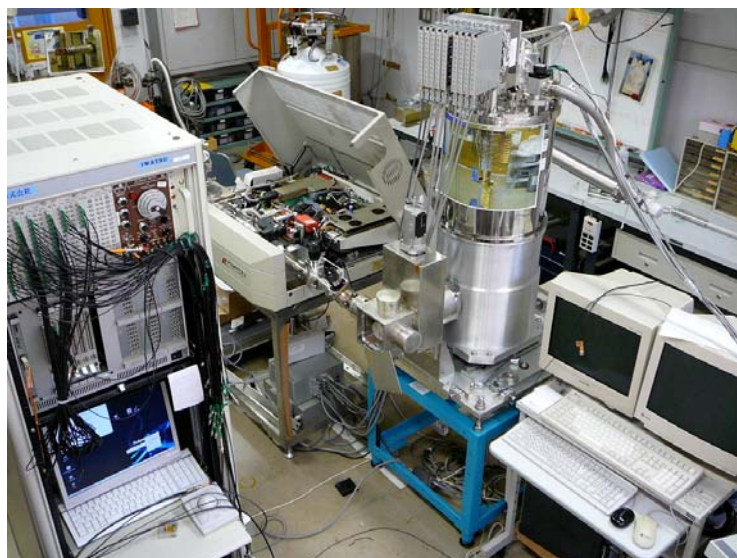
Fig. 2 Mass spectrometer for biomolecule analysis equipped with a superconducting molecule detector, a cryogen-free cryostat, and a signal process system
