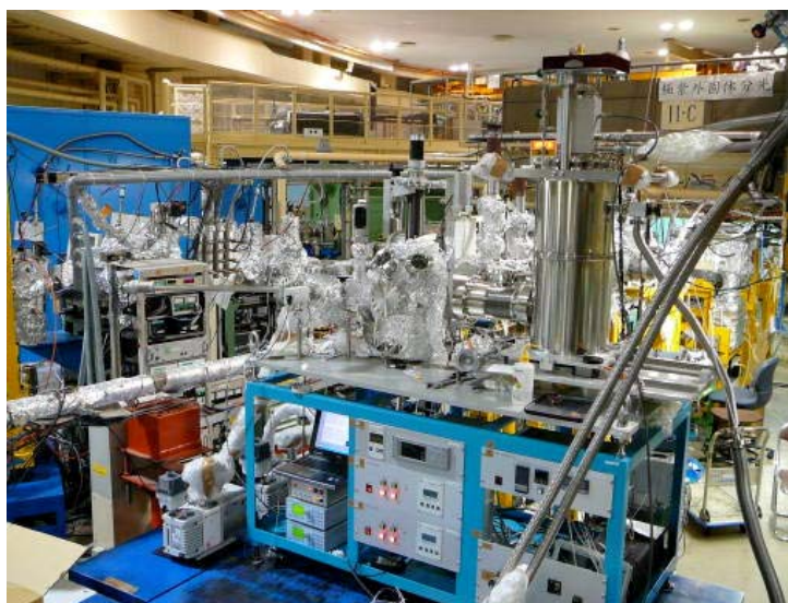
Fig. 1 Fluorescence yield XAFS spectroscopic instrument for light elements equipped with superconducting detectors
