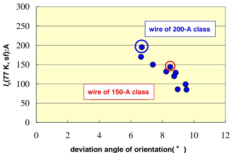
Fig. 2 Relationship between degree of crystal orientation and critical-current characteristics
