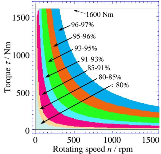
Fig.1 Example of analysis of efficiency map for HTS-ISM of 50-kW class<sup>6)</sup>
