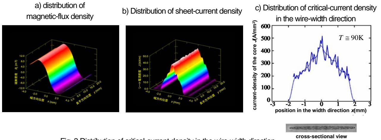
Fig. 3 Distribution of critical-current density in the wire-width direction
