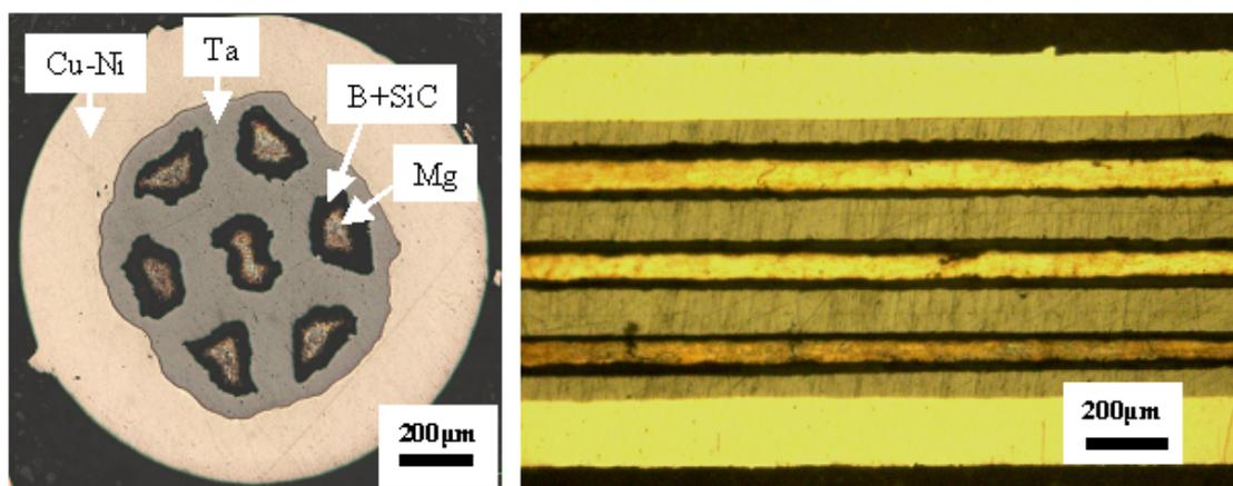
Fig. 1 Transverse section and longitudinal section of MgB<sub>2</sub> wire fabricated by internal Mg diffusion (IMD) method (before heat treatment)<sup>3)</sup>
