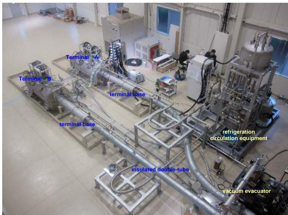
Fig. 1 Layout inside the laboratory
