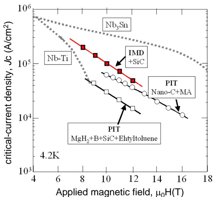
Fig. 2 Representative critical-current density ( $J_c$ )—magnetic field ( $H$ ) curve of PIT wire<sup>4),5)</sup> and IMD wire<sup>3)</sup>. Curves of Nb-Ti and Nb<sub>3</sub>Sn are shown for reference.
