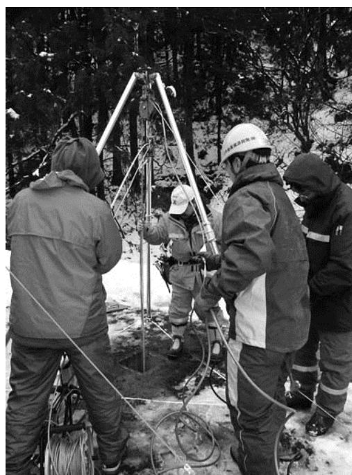
Fig. 2 Injection of the SQUID magnetometer into a trial borehole containing a steel pipe casing
