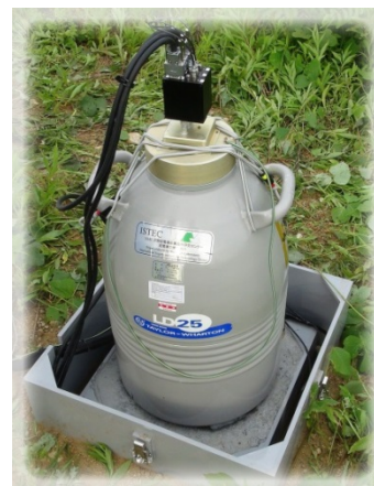
Fig. 3 HTS-SQUID magnetometer for terrestrial magnetism observation studies
