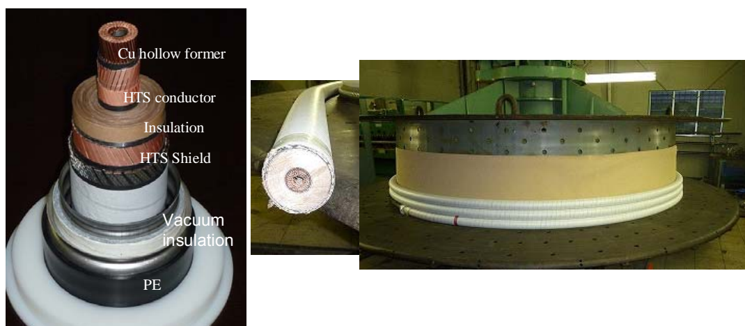
Fig. 1 The structure and outline of 275kV-3kA YBCO superconducting cable
