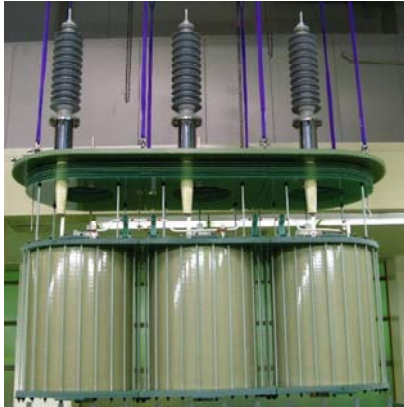
W-phase V-phase U-phase Fig. 5 2MVA-class superconducting transformer wire winding
