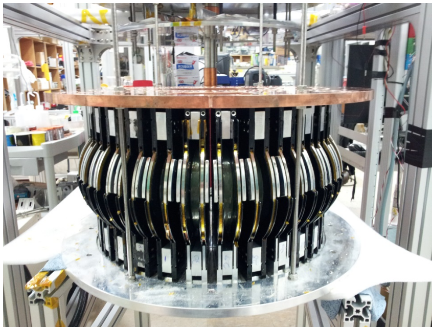
Fig. 2 Photo of 400mA 400A class DC reactor HTS coil
