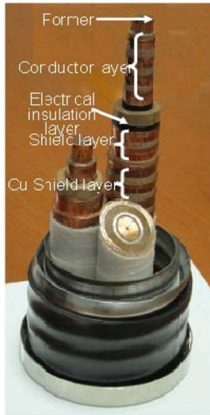
Fig.1 Large current cable (Three-in-one)
