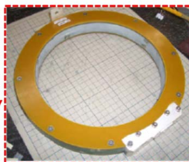
Coil current transport 1,500 A (max power output at power supply) @ 8 T
