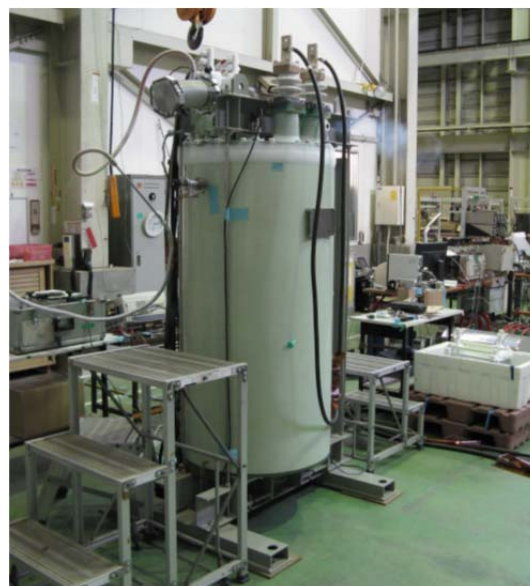
Fig. 2 Testing of a 2 kA-class large current winding
