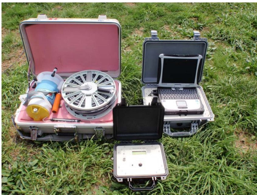
Fig. 4 SQUITEM unit 3 under development. SQUID magnetometer in the left corner, with the receiver system shown on the right, and a GPS synchronous clock in the forefront
