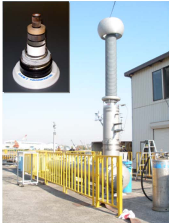
Fig. 2 The 275 kV superconducting cable model and the outdoor termination.
