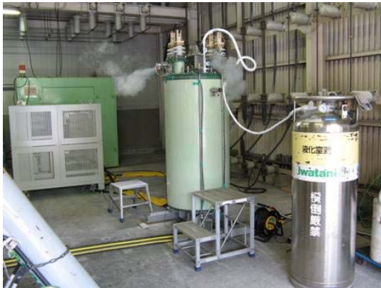
Fig. 4 A view of the test equipment used to determine the current limiting characteristics of the 400 kVA transformer.
