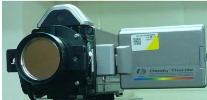
Fig. 2 The NEC bolometer-type THz Camera 12) .
