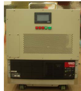
Fig. 3 Superconducting hybrid filter unit for 9 GHz band weather radar applications
