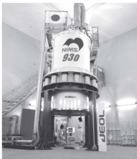
Fig. 5 A world class superconducting 1 GHz-NMR at NIMS, which survived the Great East Japan Earthquake of 11 March 5)
