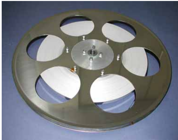
Latest Gd123 superconducting wire that was manufactured
