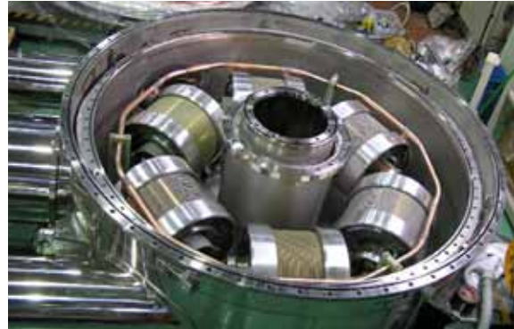
Fig. 3 Superconducting coil housed in its casing
