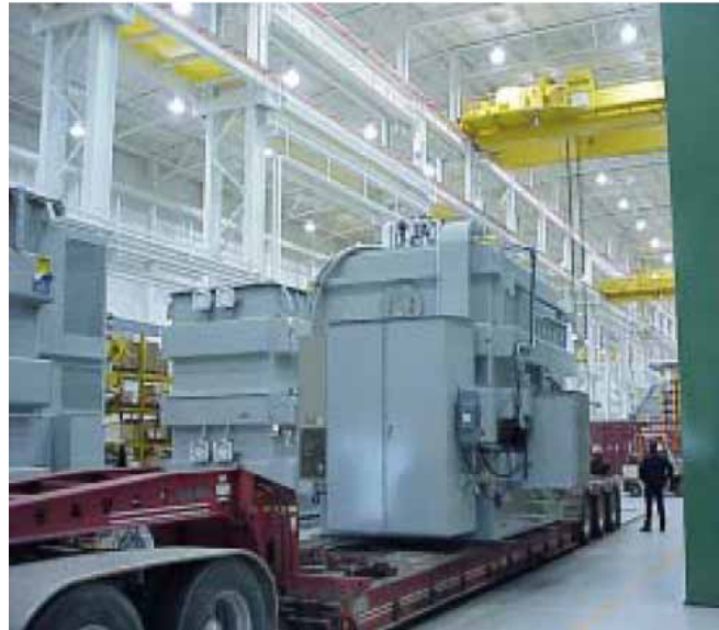
Fig. 1 A 3 \phi 24.9-kV/4.2-kV, 5/10 MVA prototype transformer manufactured by WES. The transformer is housed in a steel tank.
