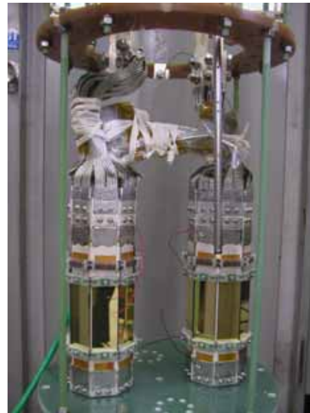
Fig. 1 Photo of 1 kA-class SFCL element
