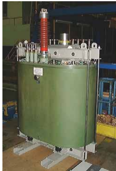
Fig. 3 A Railway Technical Research Institute prototype 1 \phi 25-kV/1.2-kV/0.4kV, 4 MVA transformer for bullet trains
