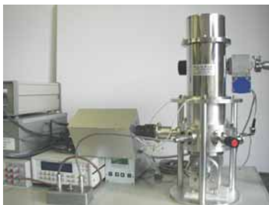
Fig. 1 Prototype liquid helium-free Josephson voltage standard system built by AIST
