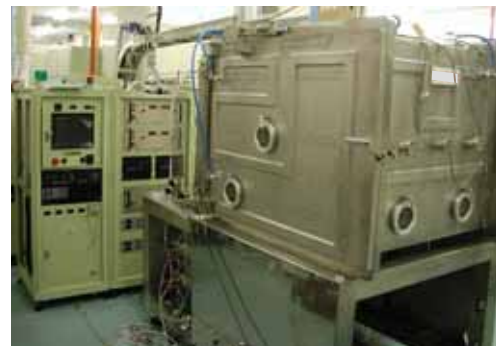
Fig.: Strong magnetic field sputtering system (actual test model)
