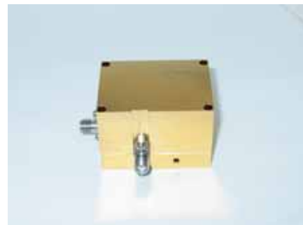
Fig. 1 4 GHz band superconducting high-power filter
