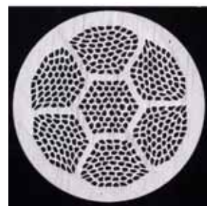
Fig. 1 Section of Bi-2212 round wire
