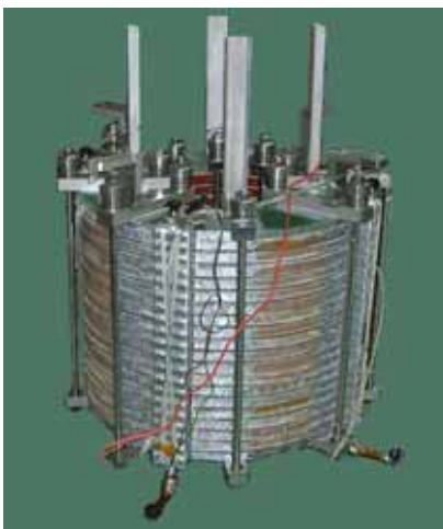
Fig. 1 1 MVA class SMES coil for bridging instantaneous voltage drops
